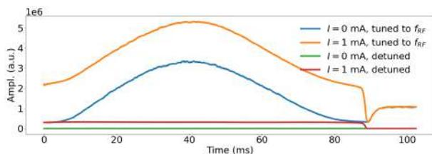
Figure 1: Measured amplitude on one channel of a Booster Spark when tuned to the RF frequency (blue, orange) and when it is detuned to a revolution harmonic of the RF frequency (green, red).
