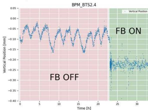
Figure 3: Orbit stability in the vertical plane at the last BPM of the BTS.
