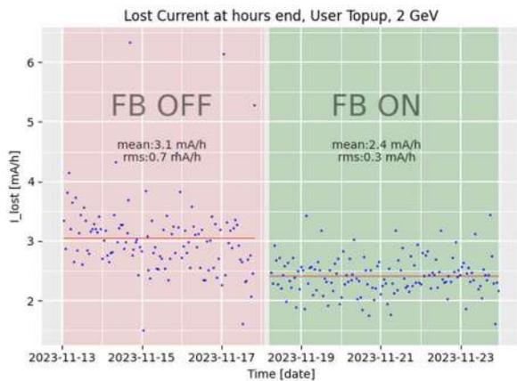
Figure 4: Improved injection efficiency after trajectory correction using the feedback.
