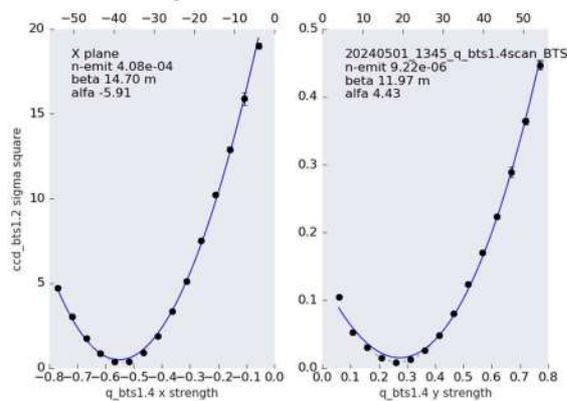
Figure 5: Example of emittance measurement by quad scan method.
