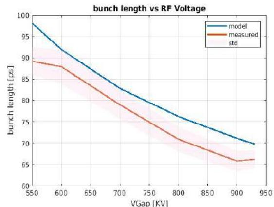
Figure 2: model vs measured bunch length.
