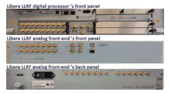
Figure 2: Libera LLRF system: digital processor's front panel (on top), analogue front-end's front panel (in the middle), analogue front-end's back panel (bottom).
