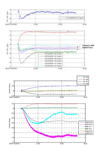
Figure 11: The upper plotis BPM/XBPM position drift when applying XBPM local feedback. The BPM drift included in the feedback loop is much smaller than those excluded in the loop. XBPM drift is also decreased from 10~14 um to 2 um. The lower plot is the fast correctors (FOFB) and ID correctors (XBPM local feedback) strength variations.
