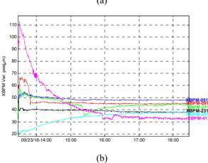
Figure 3: (a) The vertical position change of BPM nearby IDs during the first 5 hours of beam stored. (b) The vertical position change of XBPM during the first 5 hours of beam stored.
