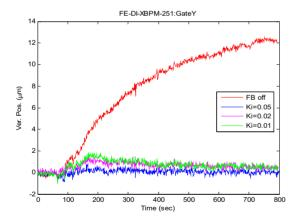
Figure 6: XBPM position drifts for different Ki coefficient.
