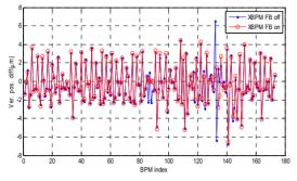
Figure 10: The overall BPM orbit drift comparison between XBPM local feedback on and off. The BPM position drift could be suppressed lower than submicron when the of this work must assigned BPM (BPM index 86-88) included in the feedback loop.
