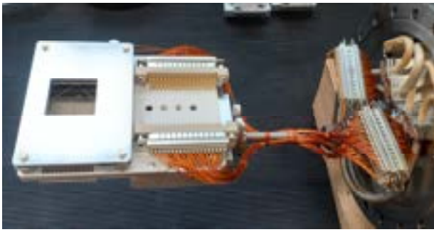
Figure 3: SEM harp by PROACTIVE. The grid consists of two harps rotated by 90°, area 32 mm x 32 mm with diamond shaped cleaning electrode, 64 wires per harp, wire pitch 0.5 mm, thickness 100 \mu\text{m} .
