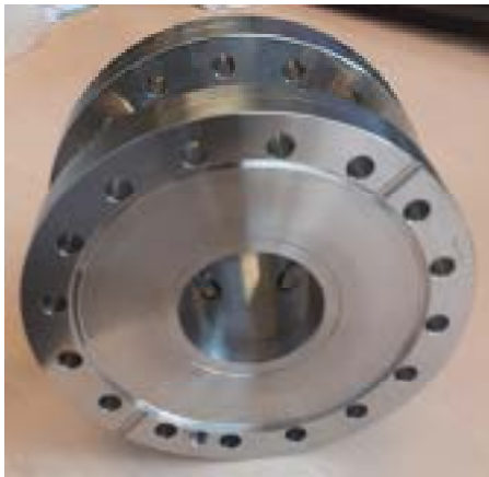
Figure 4: Beamline BPM by NTG. Aperture 50 mm, button diameter 12 mm, total length 80 mm, DN100CF.
