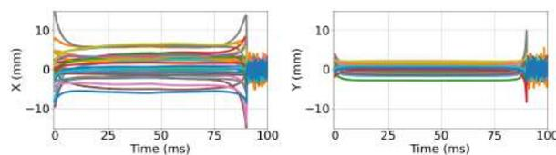
Figure 5: Uncorrected orbit distortion at all 31 BPMs.
