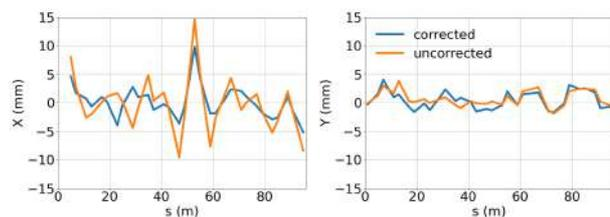
Figure 6: Closed orbit distortion at injection energy.
