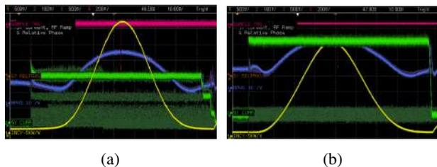
Figure 3: Beam current (green curve) in the original state (a) and after tune and chromaticity corrections, with higher current and beamloss at lower energy on the downramp (b).
