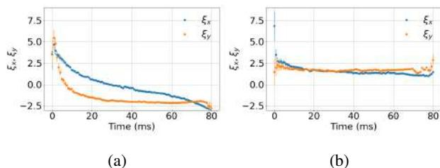
Figure 4: Measured chromaticity during the acceleration ramp in the original operational state (a) and after correcting to a nearly-constant, slightly positive value (b).
