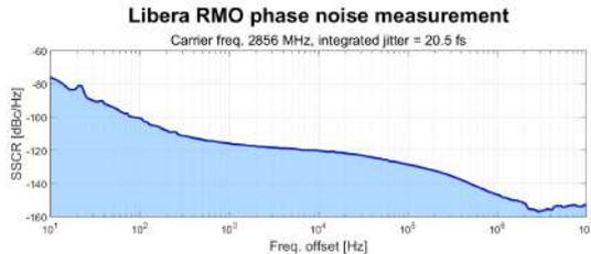
Figure 4: Integrated phase jitter of the RMO, measured with a Rohde&Schwarz FSWP-26 phase noise analyzer (between 10 Hz and 10 MHz from the carrier).
