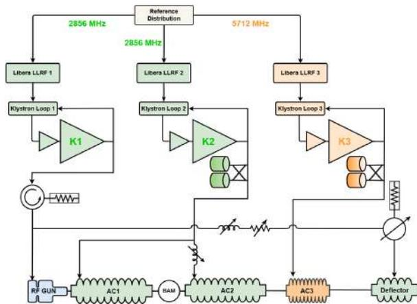
Figure 1: Block diagram of the SPARC\_LAB LLRF system.
